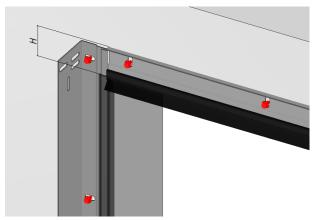
TOP PROFILE TO BE MOUNTED PRECISELY ON THE LEVEL OF THE VERTICAL ANGLE CUT THE SEAL ON THE VERTICAL ANGLE FROM THE TOP H=65mm ASSEMBLY THE TOP SEAL ON THE TOP PROFILE THE SEAL OF THE SAME LENGTH!
