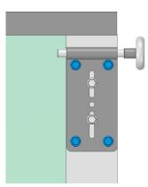
AFTER ADJUSTMENT TIGHTEN THE BRACKET WITH THE BOLTS
