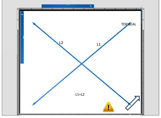
BEFORE TIGHTENING CHECK ALL VERTICAL AND HORIZONTAL ADJUSTMENTS AND LENGTHS OF DIAGONALS L1=L2
