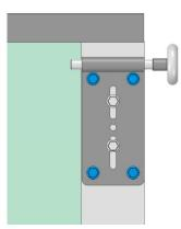
AFTER ADJUSTMENT TIGHTEN THE BRACKET WITH THE BOLTS **OPTION:**
